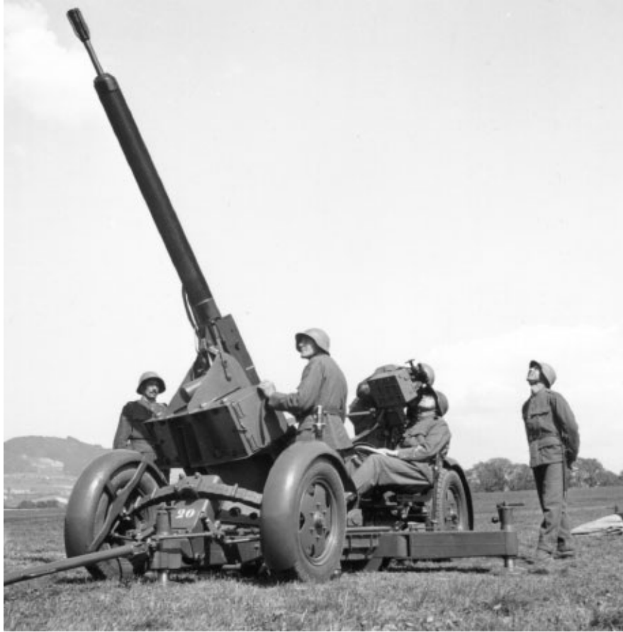
This Swiss-made 20mm anti-aircraft gun fired 250 rounds per minute with a range of 4,500 meters.
