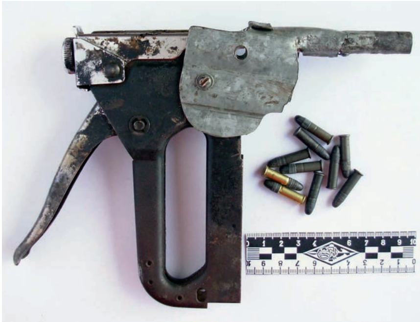
Image 22 A staple gun adapted to fire .22 LR ammunition, with the addition of a length of tubing for a barrel
