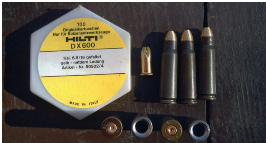
Image 19 Improvised ammunition made from 7.62 × 39 mm cartridge cases modified to accept 6.8 mm Hilti powder-actuated tool cartridges in place of a primer and loaded with a projectile turned from brass bar. This hybrid ammunition is designed for use in an improvised ‘sub-machine gun’
