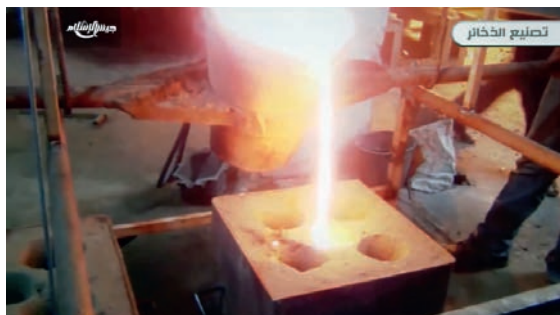
Image 8 Jaish al-Islam uses the sand casting technique to produce mortar projectile bodies, 2014
